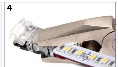
4 Complete the LED Strip connections using pliers. Make sure connection is locked at base of connector
