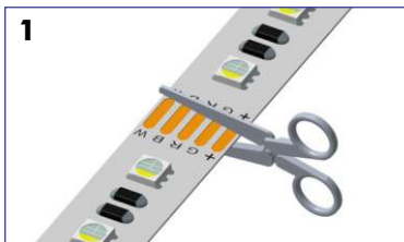
1 Cut the LED Strips at the cut mark (pads)
